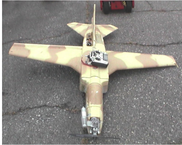
Fig. 7 Mig 117 Bravo modified target drones were equipped with modern engine and Micro-Pilot autopilot.
